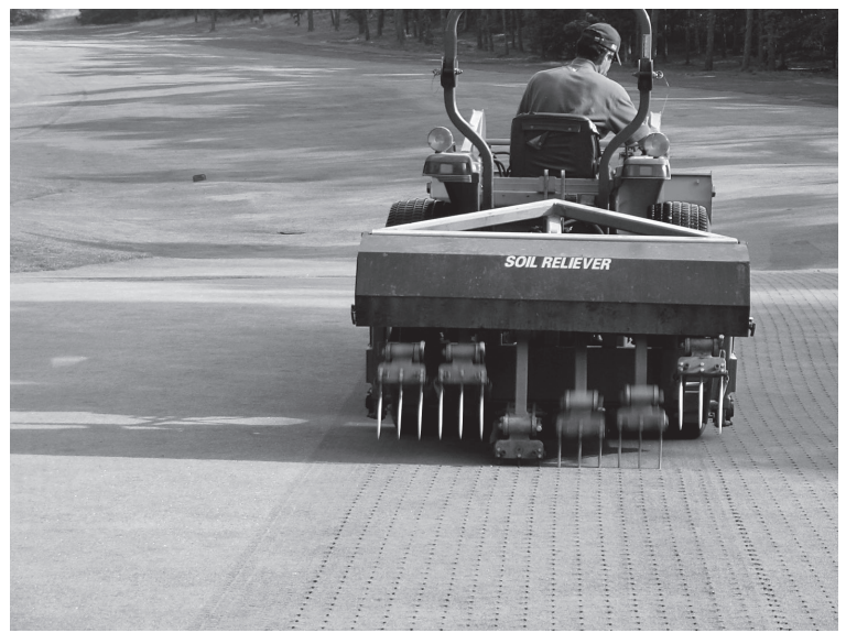
Aerating the greens with a machine that leaves plugs. This is done to loosen compacted soil to make more room for and increasing oxygen to the roots. It usually takes a couple weeks for the holes to fill in and grow over.
