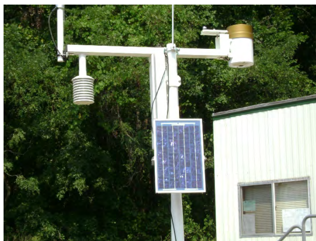
Figure 10. Onsite weather stations can provide potential ET data to help determine irrigation needs.
