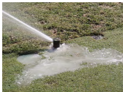
Figure 8. Leaky o-ring identified during routine inspection.
