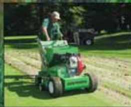
Graden with Sand Injection
