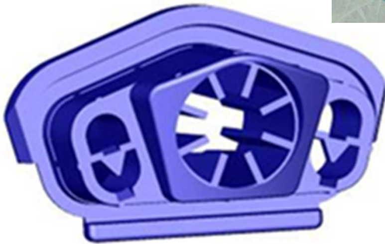
Penta Nozzle Design of the Rain Bird 751
