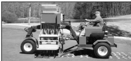
Drill / Backfill Aeration Bit Sizes: 3/4" x 12" or 1" x 8" Straight Drill Aeration Available
