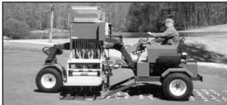
Drill / Backfill Aeration Bit Sizes: ¾" x 12" or 1" x 8" Straight Drill Aeration Available
